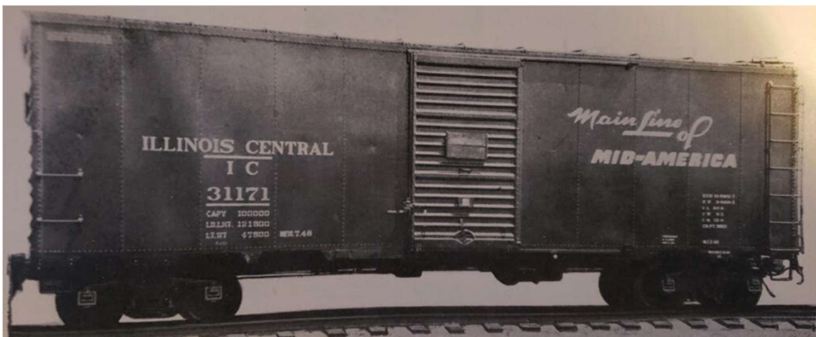
Taken from an ad for Youngstown Doors in the 1949 Car Builders Cyclopedia, car 31171 provides an example the Improved Youngstown Door used on some of the 1948 builds.
