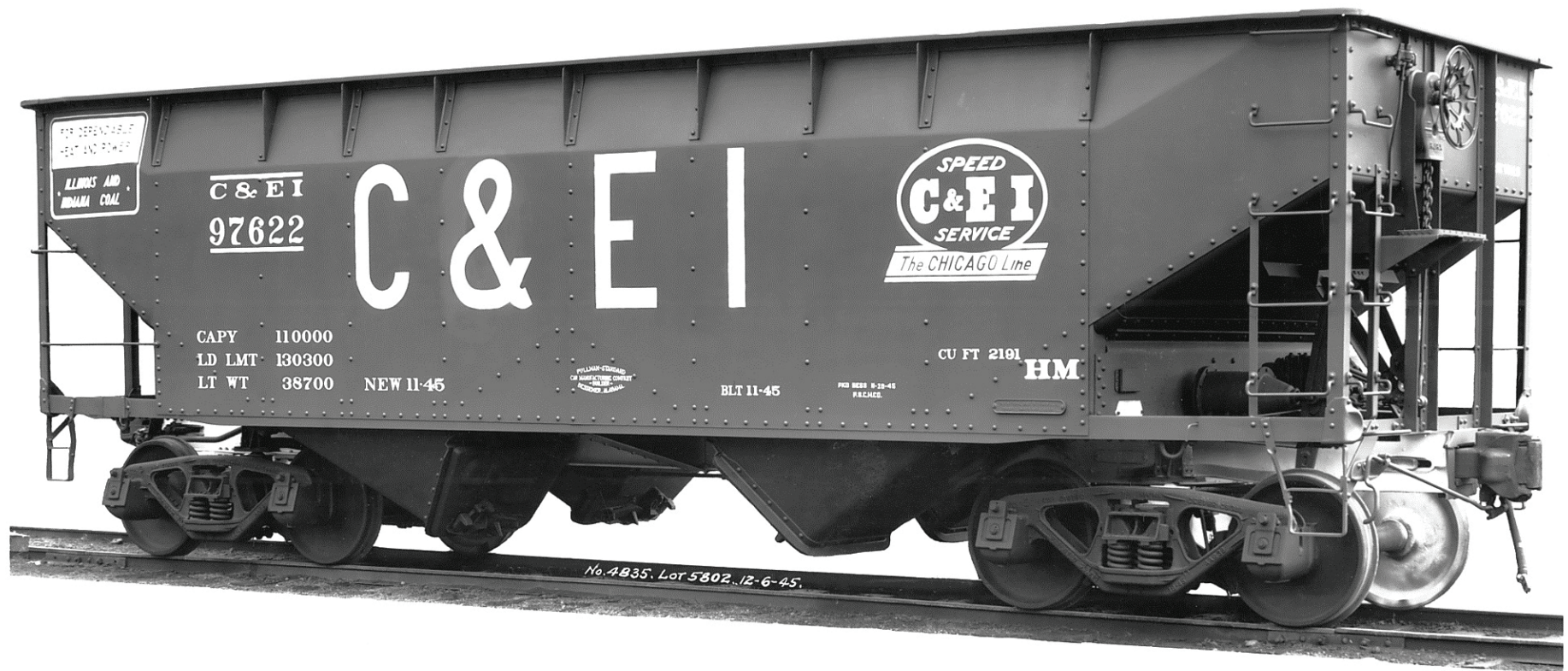
Chicago & Eastern Illinois 97622 from series 97500-97999, built November 1945 by Pullman-Standard. All cars in the series came with Ajax power hand brakes, Enterprise Unit door locks, Apex Tri-Lok brake steps, and ASF A-3 Ride-Control trucks with one-wear steel wheels. The outside of sides and ends were painted Pittsburgh #55666 Carhide Grey or Glidden Grey Steel Car Finish Coat (250 cars each). Black car cement was applied to the underframe and trucks were painted black. Stencils were white. Pullman-Standard photo, Smithsonian Institution, NMAH/Transportation, Haskell and Barker Collection, Negative 4835.
