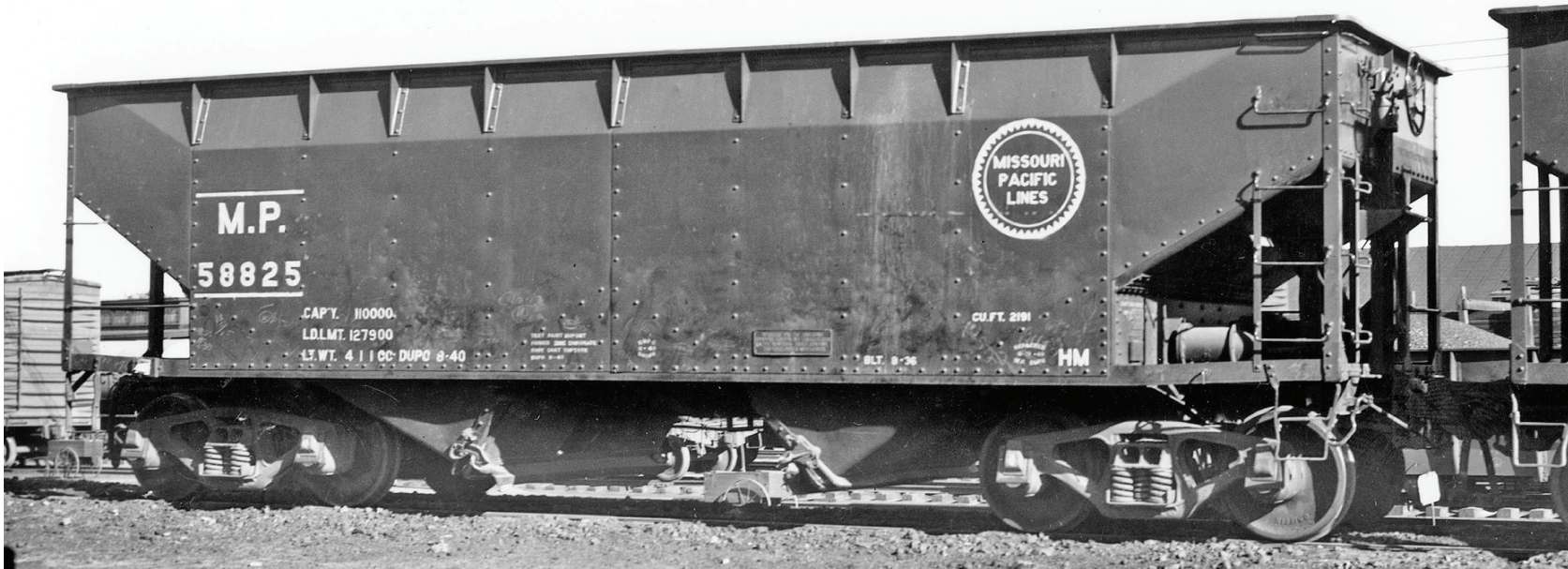
MP 58825 (series 58750-59249), built 8-36 by AC&F, reweighed Dupo, IL 8-40. MP had 2,200 nearly identical cars built by three car builders from 1936 to 1941. Missouri Pacific photo, Bill Hoss collection.
