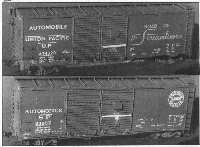
From the advent of the automobile, the railroads strove to accommodate their special needs of shipment by rail. Car heights were increased and doors widened. When racks which stacked automobiles were developed, the railroads quickly adopted them to increase auto density. Auto traffic represented a prized lading worth extra competitive
